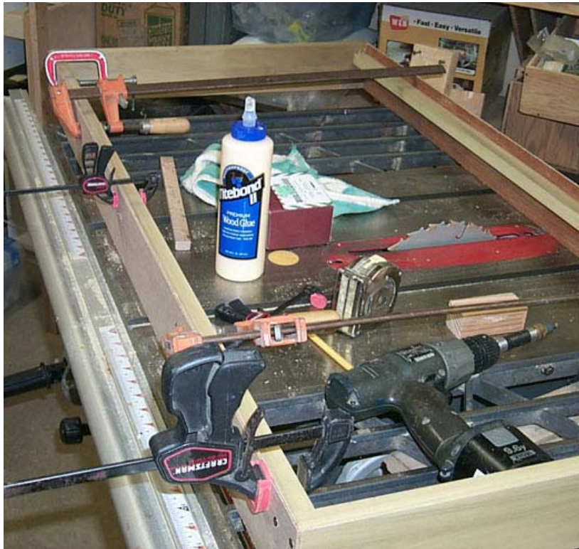
1 1/8" Stiffeners are ripped from 1 X 4 poplar, glued and screwed to sides and ends to form a T girder, serve as a ledge for the foam top as well as stiffen the sides.
