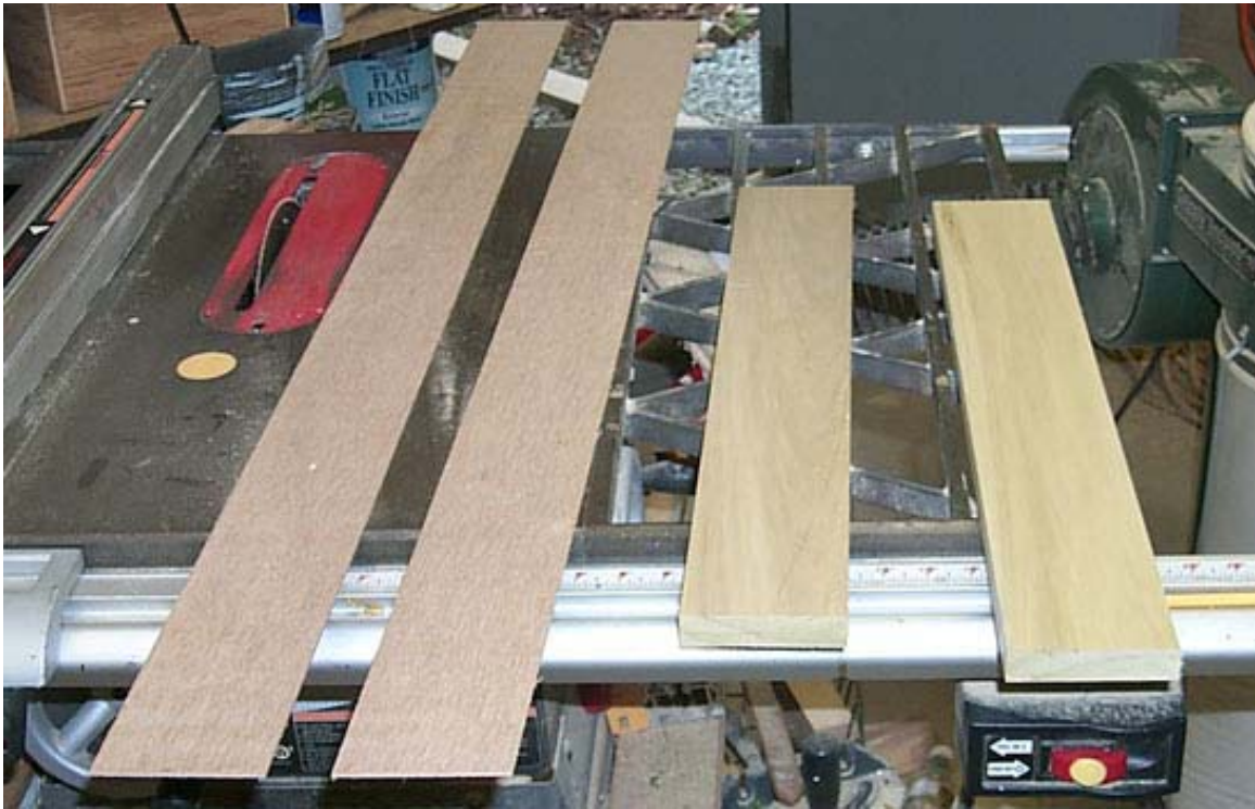
Lightweight sides are cut from 1/8" luan plywood and ends are cut from 1 X 4 Poplar.
