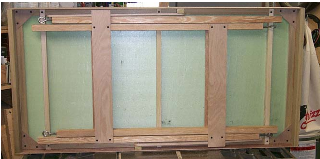
The second pair of legs is attached. Note that this set of legs has extended braces, mounted on the front side of the legs, so that the captive diagonal braces will be secured when the legs are folded.
